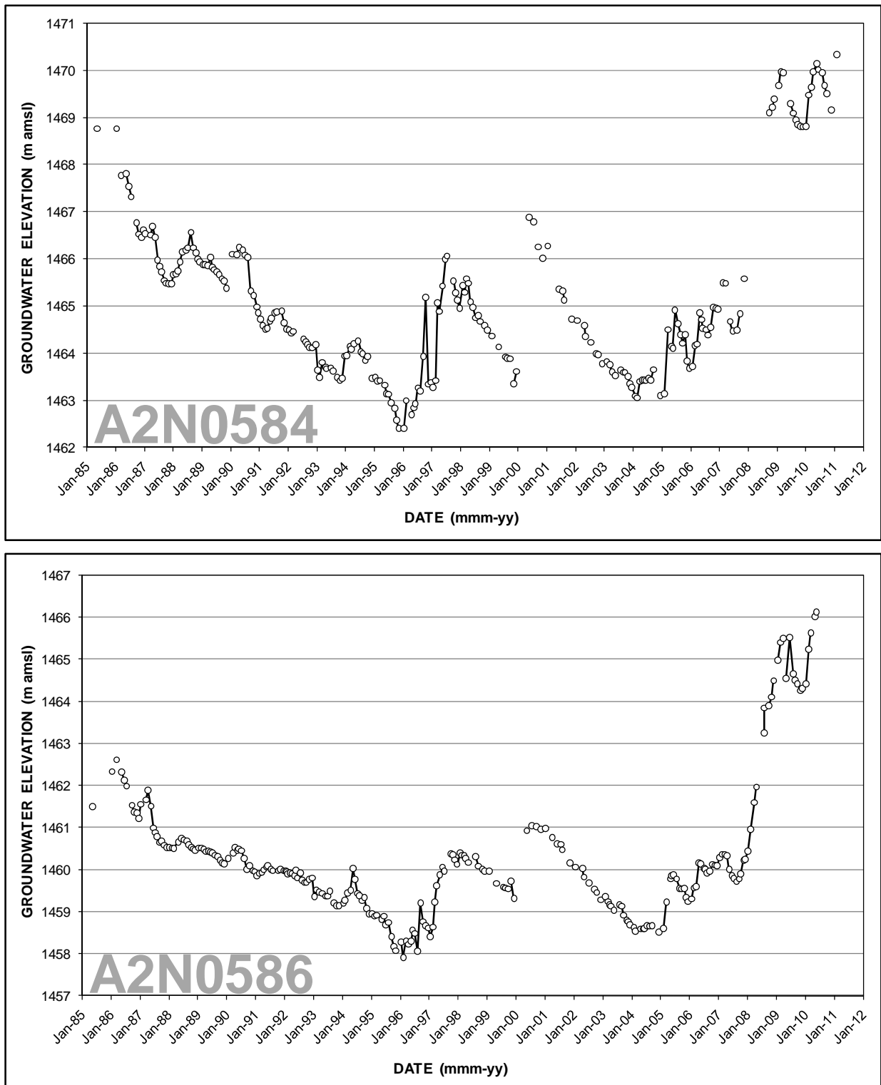
Figure 1. Hydrographs of two DWA long-term water level monitoring boreholes (stations A2N0584 and A2N0586) upstream of Sterkfontein Caves. See Maps 1 and 2 for positions of these stations.
